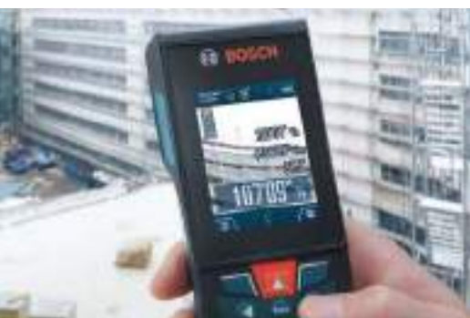
Camera for optimum visibility of laser point at a distance of 150 m
